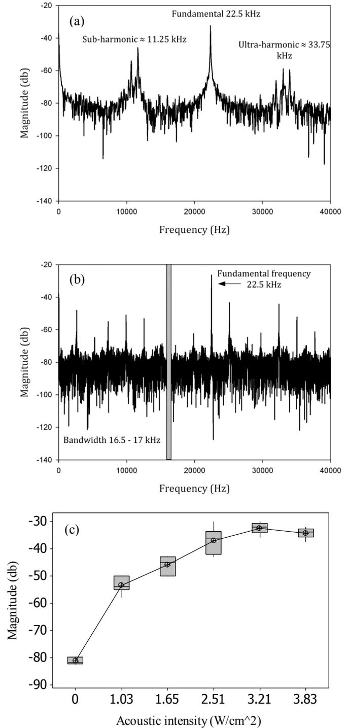
Fig. 4. (a) Acoustic spectrum of waveguide operating at  $1.65 \text{ W/cm}^2$  (b) Acoustic spectrum of waveguide operating at  $3.21 \text{ W/cm}^2$  (c) Acoustic broadband noise versus acoustic intensity for bandwidth of 16.5-17 kHz in FFT spectrum.
