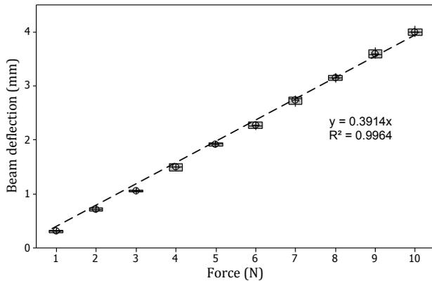
Fig. 3b. Calibration of the cantilever beam: Beam deflection versus applied force at wire waveguide point of entry ( $n = 6$ ).
