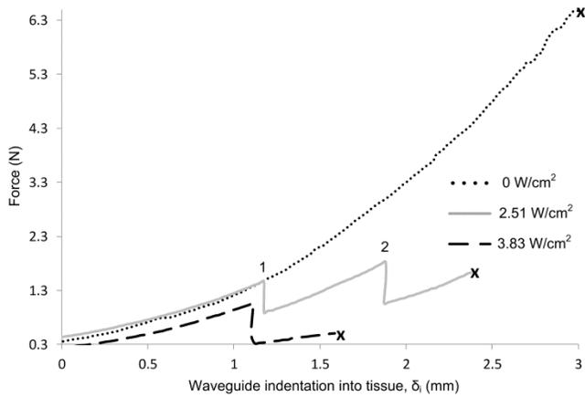
Fig. 5. Force versus distal tip indentation into tissue,  $\delta_i$ , profiles for individual tests, for a range of acoustic intensities. Note: Non-energized is depicted as 0 W/cm<sup>2</sup>.
