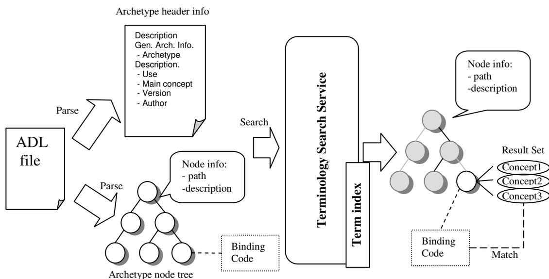
**Figure 2:** General process of constructing a Shadow from Archetypes
