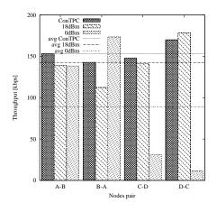
Figure 11: Throughput observed in 4 nodes case
