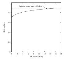
Figure 2: Delivery ratio vs. TX power characteristics for a high quality link
