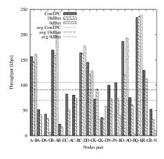
Figure 12: Throughput observed on 11 node testbed
