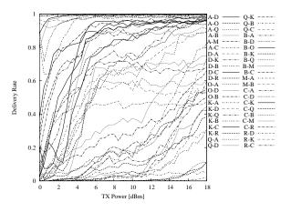
Figure 5: Delivery rate vs TX power
