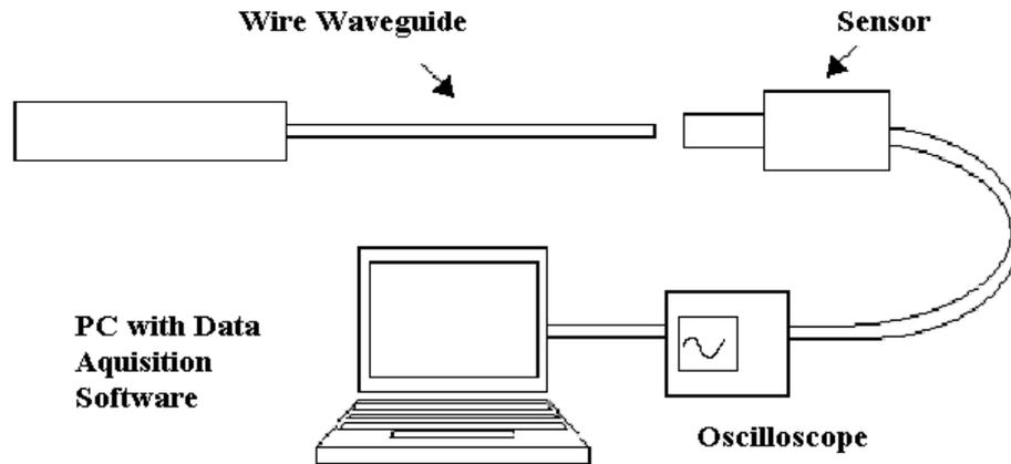
**Figure 1:** Wire waveguide displacement measurement set up with laser sensor, hardware low band pass filter and PC with data acquisition software
