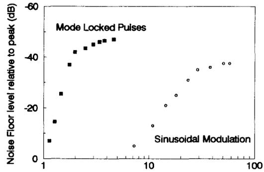
Fig. 2. Noise floor level relative to peak level of the synchronized self-pulsing laser output signal as a function of the injected optical power for mode-locked and sinusoidal input signals.
