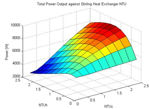
Figure 6. Total Power Vs Heat Exchanger NTU
