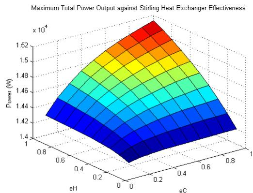
Figure 8. Total Power Vs Heat Exchanger  $\epsilon$
