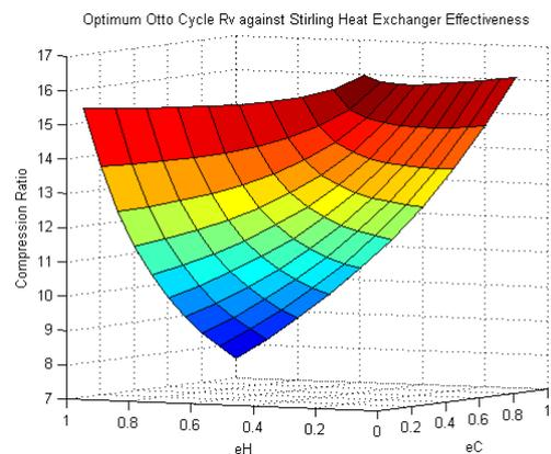
Figure 10. Otto Cycle Optimum Compression Ratio Vs Heat Exchanger  $\epsilon$
