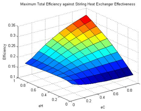
Figure 3. Total Efficiency Vs Heat Exchanger  $\epsilon$
