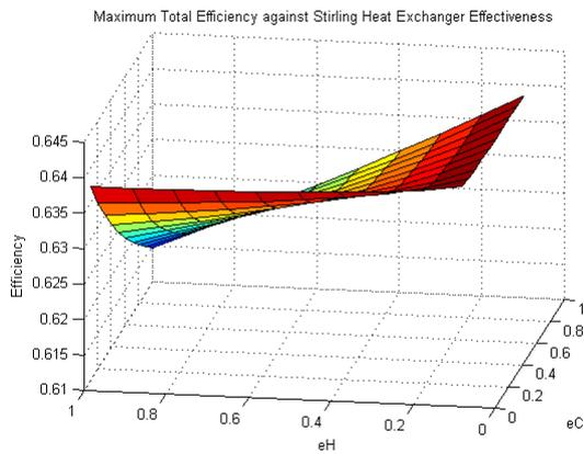
Figure 9. Total Efficiency Vs Heat Exchanger  $\epsilon$
