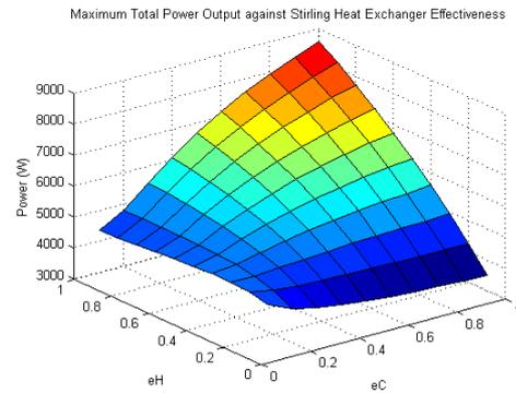
Figure 2. Total Power Vs Heat Exchanger  $\varepsilon$
