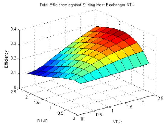
Figure 7. Total Efficiency Vs Heat Exchanger NTU
