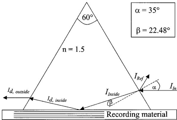
**Fig. 10** Replay geometry, illustrating the Fresnel boundary reflections.
