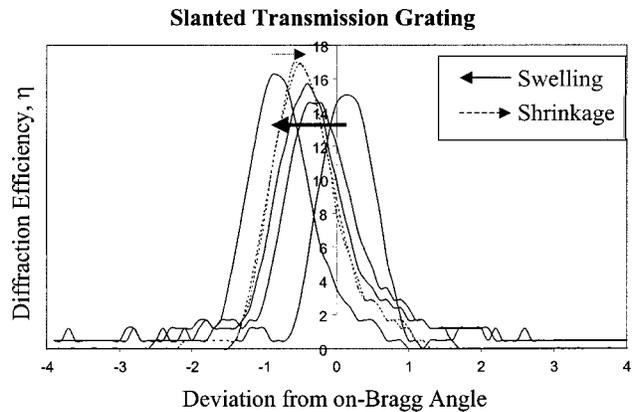
**Fig. 2** Variation in on-Bragg replay angle due to material thickness variations. Initial thickness=120±10  $\mu\text{m}$  (micrometer screw gauge), initial slant angle=25 deg, initial spatial frequency = 1000 lines/mm,  $\lambda = 633 \text{ nm}$ .
