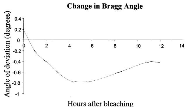
**Fig. 3** Change in the Bragg angle for a slanted transmission hologram due to thickness changes caused by the bleaching process. Initial thickness=120  $\mu\text{m}$ , initial slant angle=25 deg, initial spatial frequency=1000 lines/mm.
