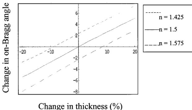
**Fig. 7** Change in replay angle as a function of thickness for three different refractive index values. Here  $n_{av} = 1.425$ , 1.5, and 1.575,  $\theta_B = 34$  deg,  $\lambda = 633$  nm, slant angle  $70^\circ$ .
