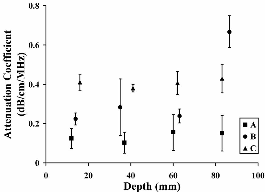
**Figure 3.** Variation of attenuation coefficient (dB/cm/MHz) as a function of depth (cm) in phantoms A, B and C with phantom A containing no Al<sub>2</sub>O<sub>3</sub> scatterers, phantom B containing 0.88 wt% of 0.3 µm Al<sub>2</sub>O<sub>3</sub> and 0.94 wt% 3 µm Al<sub>2</sub>O<sub>3</sub>, and phantom C containing 2 wt% 0.3µm Al<sub>2</sub>O<sub>3</sub>, respectively.
