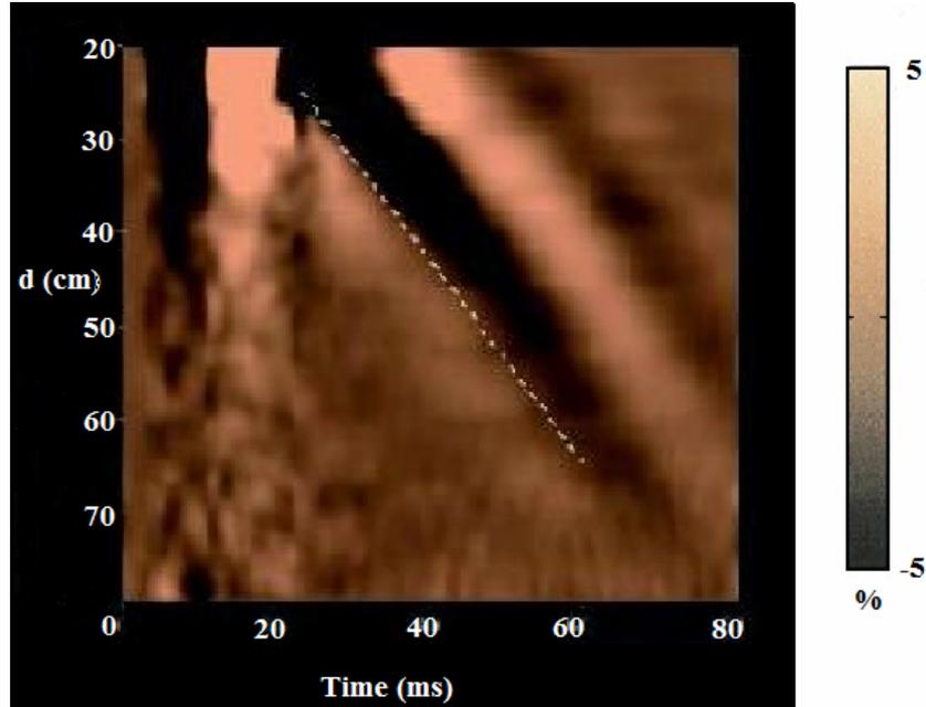
**Figure 2.** Example of an elastogram measured by the Fibroscan® system, displaying the amplitude of the strains induced in a healthy patient liver as a function of depth ( $d$ ) and time. The stiffness measurement is derived from the velocity of the shear wave propagated in the liver tissue.
