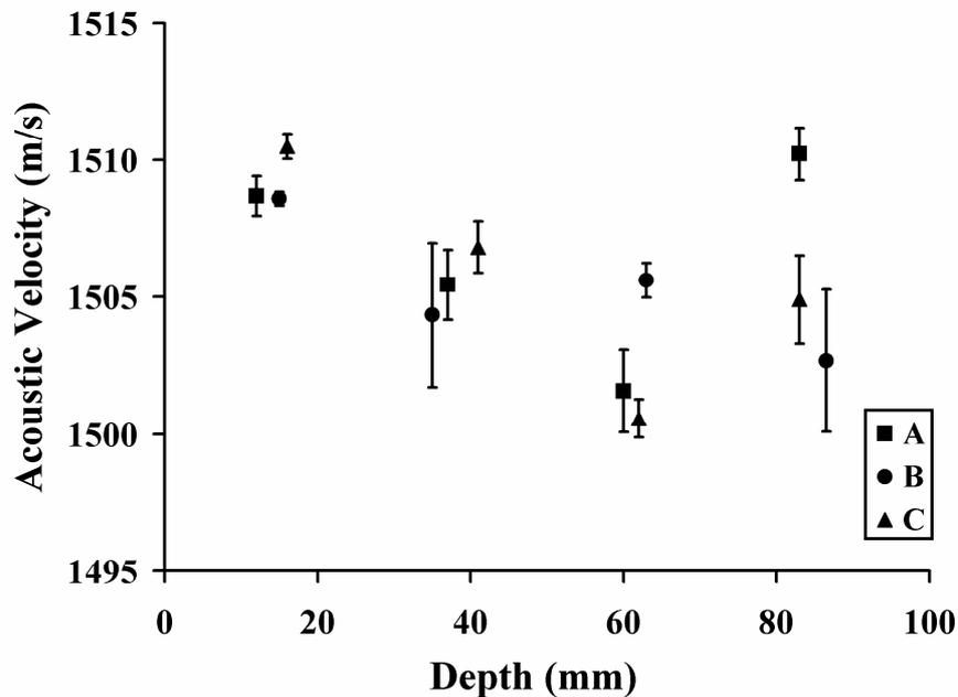
**Figure 4.** Variation of acoustic velocity (m/s) as a function of depth (cm) in phantoms A, B and C with phantom A containing no  $\text{Al}_2\text{O}_3$  scatterers, phantom B containing 0.88 wt% of 0.3  $\mu\text{m}$   $\text{Al}_2\text{O}_3$  and 0.94 wt% 3  $\mu\text{m}$   $\text{Al}_2\text{O}_3$ , and phantom C containing 2 wt% 0.3 $\mu\text{m}$   $\text{Al}_2\text{O}_3$ , respectively.
