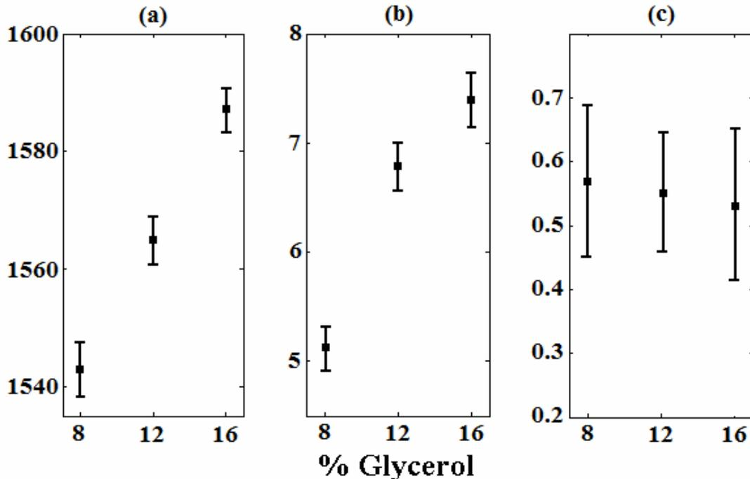
**Figure 5.** Effect of glycerol concentration on (a) the acoustic velocity (m/s), (b) Young's modulus values (kPa), and (c) attenuation coefficient (dB/cm/MHz) for 6 % PVA-C samples processed through 4 freeze-thaw cycles.
