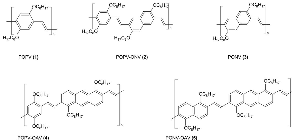
Fig. 1. Polymer structures 1–5.
