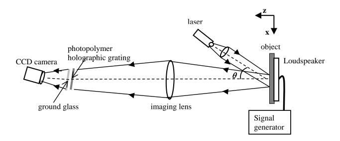
Fig.2. ESPSI system for vibration measurements with one photopolymer grating
