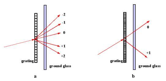
Fig.4. Propagation of the beams through the shearing device of holographic grating and ground glass: a) grating with smaller spatial frequency; b) grating with bigger spatial frequency
