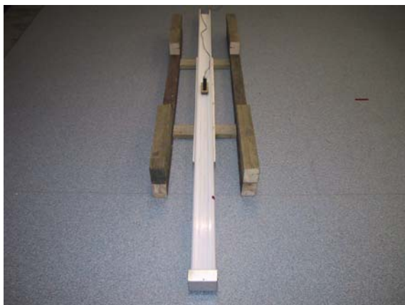
Figure 5 The frame on which the spinal board rests during measurement of spinal curvature. The motor draws the magnetometer trolley along the plastic track by means of a thin nylon cord.
