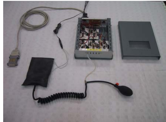
Figure 3 The pressure measurement apparatus. Here, only one of the five pressure measurement sacks is connected to the unit housing the instrumentation amplifiers.
