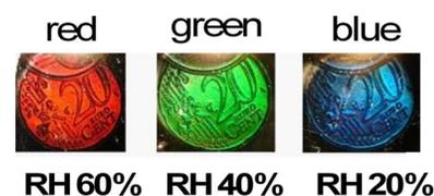
FIG. 3. (Color online) Color appearance of a hologram exposed to different humidity levels.
