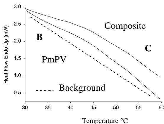
**Figure 1(b).** Thermogram of the SWNT Composite showing high temperature region
