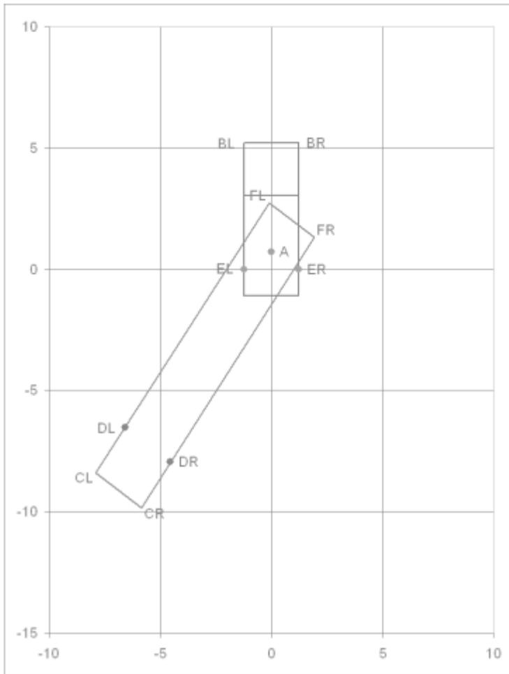
**Figure 4** Diagram from the Paths sheet showing the path of an articulated truck to scale. The truck left a testing lane that had a specified width and did a U-turn. The closest front- and sidewall positions for a minimum approach clearance of 0.2 metres were also plotted. Pressing and holding a button on the sheet caused the truck to move on this diagram.
