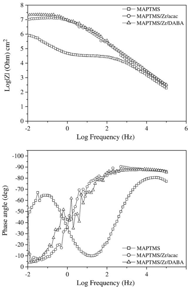
Fig. 10. Bode plots of coatings after 1 h immersion in dilute Harrison's solution.
