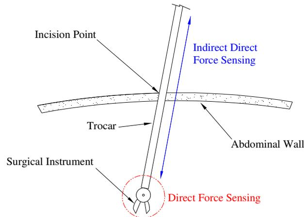
**Figure 2. Indirect and Direct Sensor Locations**
