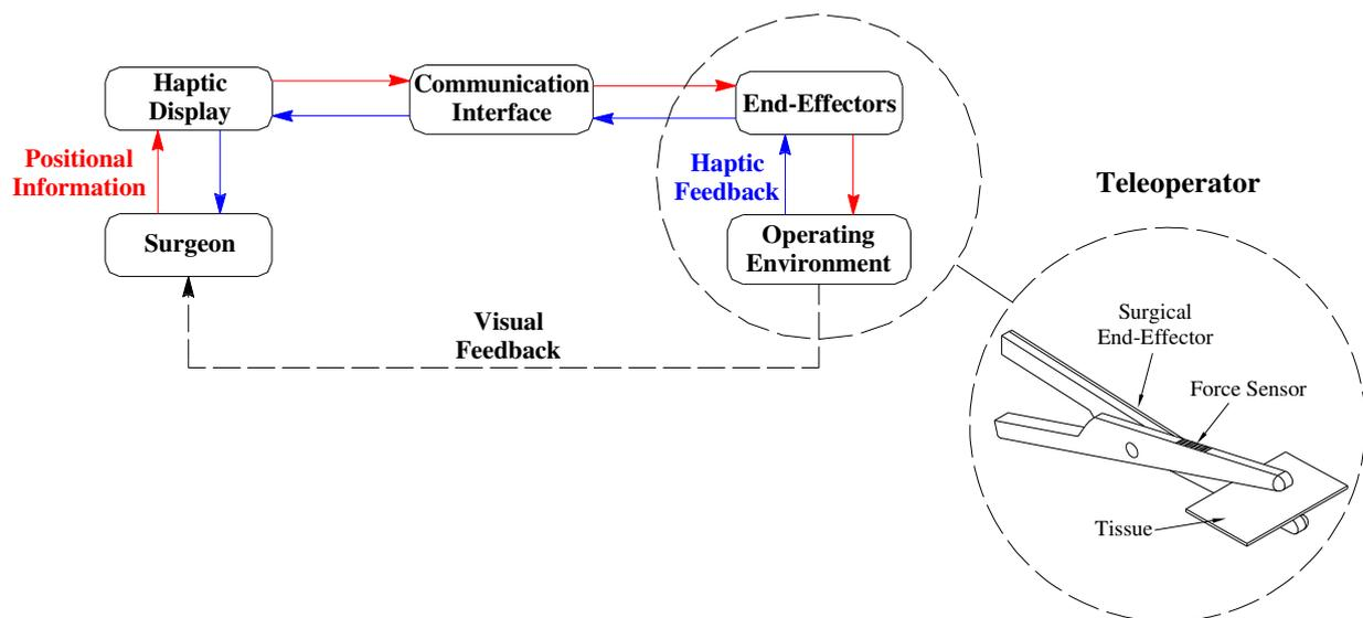
**Figure 1. Minimally Invasive Robotic Surgical (MIRS) System**
