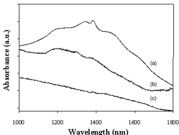
Fig.2. NIR Absorption Spectra of dropcast (a) Raw HCNT (b) Starch, Bromine, HCNT Complex (c) Starch (Note: b and c multiplied by a factor of 10)
