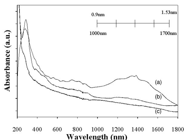
Fig.1. UV/VIS/NIR Absorption Spectra of dropcast (a) Raw HCNT (b) Starch, Bromine, HCNT Complex (c) Starch.
