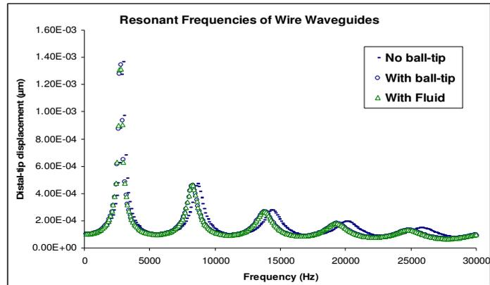
Figure 6: Numerically Determined Resonant Frequencies for waveguides
