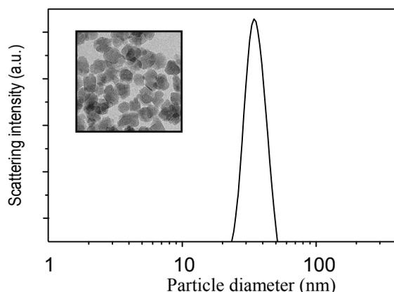
**Figure 2.** Dynamic light scattering curve of Si-MFI zeolite nanocrystals in water suspension prior mixing with photopolymer; the inset shows a TEM picture of the crystalline particles ( $M=30 \text{ nm}$ ).
