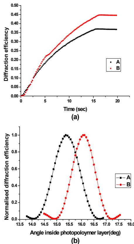
**Fig. 3** Diffraction efficiency growth (a) and angular selectivity curves (b) for gratings recorded in A- Undoped; B- Si-MFI doped photopolymer, 16sec, the corresponding peak positions in (b) are B-  $16.123^\circ$ , A-  $15.360^\circ$
